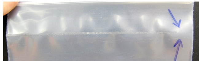
Improper Heat Seal
