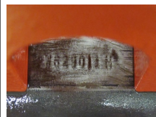
Serial number recovery using non-destructive magnetic recovery techniques
