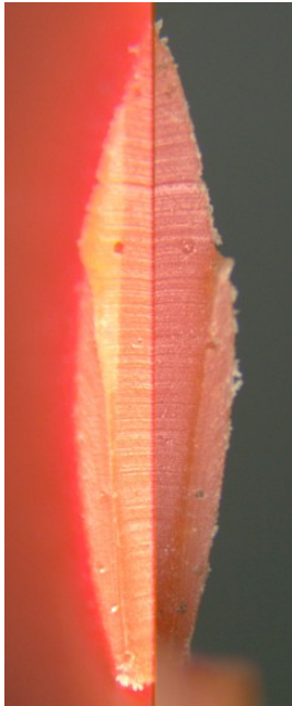
Cut extension cord insulation Evidence to evidence micro- scopic comparison
