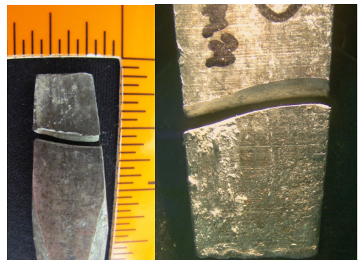
Screwdriver tip found in an object that had been pried open physically fit to a broken suspect screwdriver
