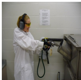
Forensic Scientist Sarah Zarnick test firing into the bullet recovery water tank
