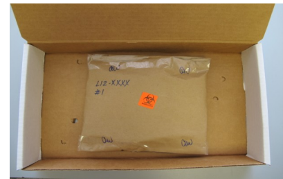
Proper use of internal, sealed/labeled packaging of contaminated items.
