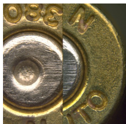
Microscopic comparison of fired cartridge case evidence.
