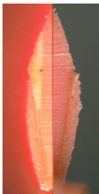
Toolmark comparison of cut marks on wire insulation.
